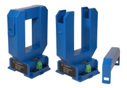
from the sensor, the relay will change state. This provides the best level of protection for critical loads. The LED indicator shows green when the sensor is powered and red when the output has tripped. With four models available the trip point can be set between 200 and 1600 amps. The adjustment is made with a potentiometer on the sensor base, with a range of 400 amps in 180 degrees of swing to the knob.
